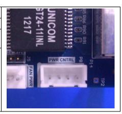
These signals can be used with +12V power supplies that provide Power Good and can utilize a Power Good signal. Power Good is an open drain signal and is pulled up to +5V on the COM Express carrier.
