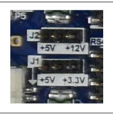
LVDS backlight enable polarity
