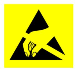
Electronic components and circuits are sensitive to ElectroStatic Discharge (ESD). When handling any circuit board assemblies including Connect Tech COM Express carrier assemblies, it is recommended that ESD safety precautions be observed. ESD safe best practices include, but are not limited to:
