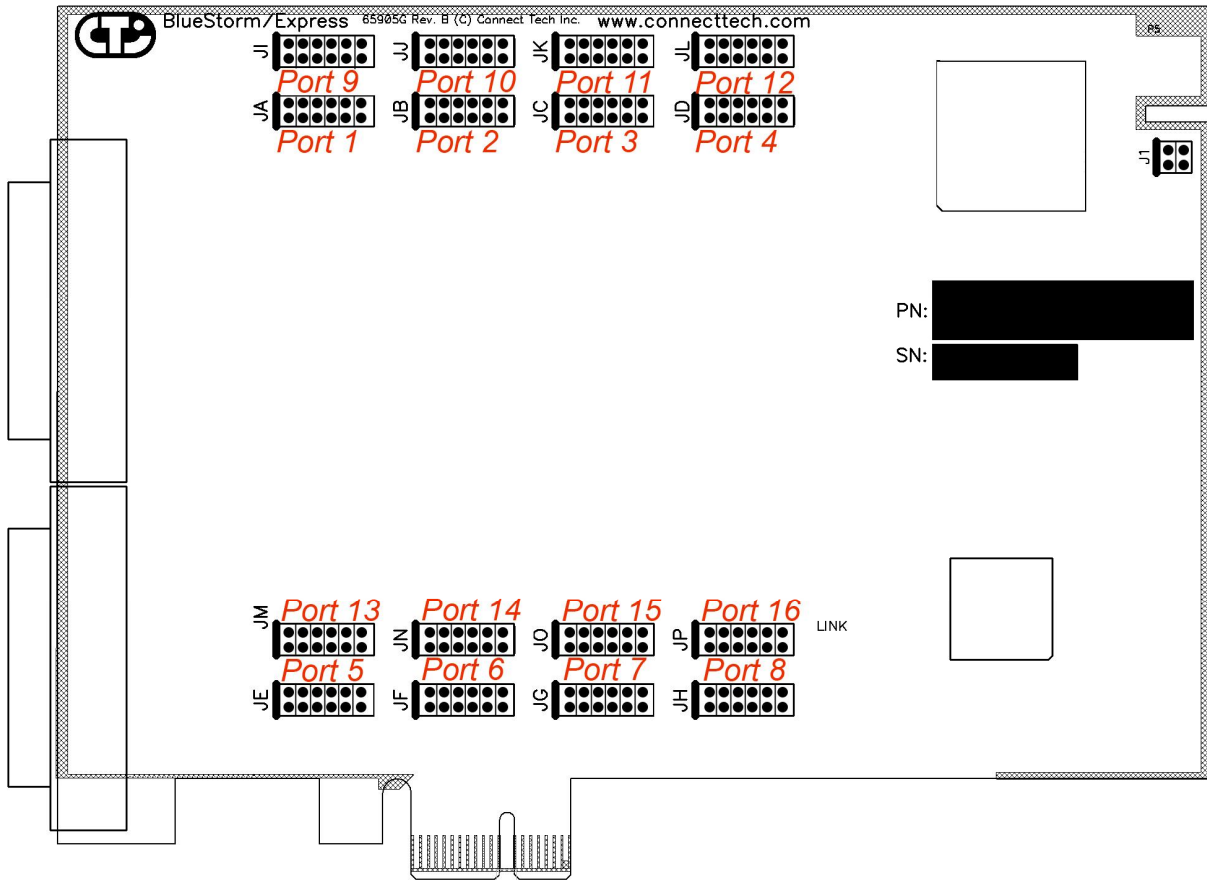
Figure 2: BlueStorm/Express RS-232/422/485 eight & 16 port models hardware components
